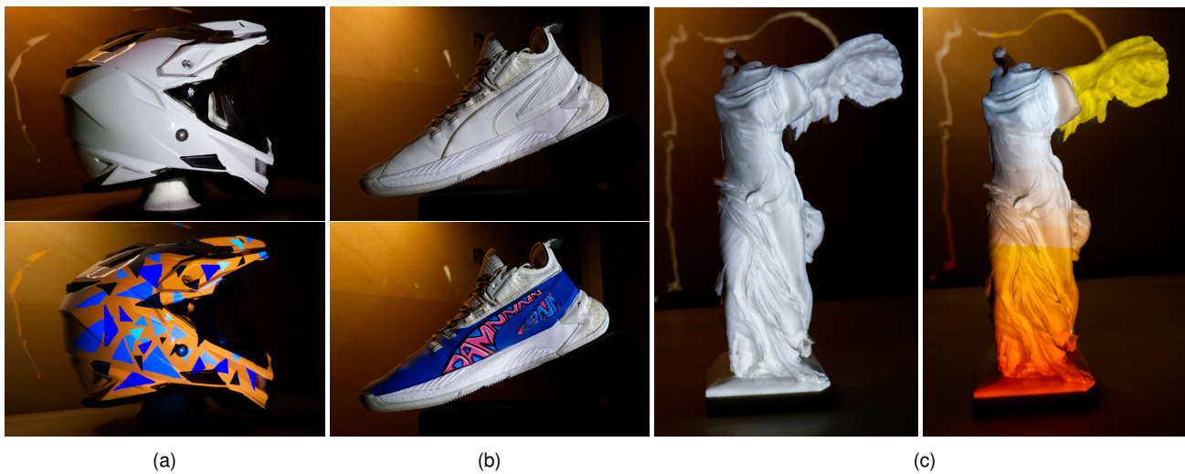
Figure 13. Projection (painting) results on (a) a motorcycle helmet, (b) a shoe, and (c) the Winged Victory of Samothrace statue. The white projections are shaded fusion results of successfully reconstructed areas.
