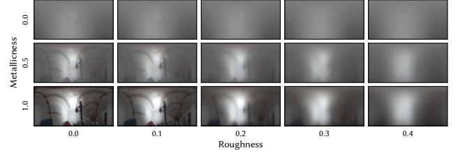
Figure 5: Environment illumination from the point of view of a material sample with the Disney Principled BRDF. With increasing roughness, the reflection lobe widens and causes blurring. With decreasing metallicness, the reflection softens and becomes diffuse.
