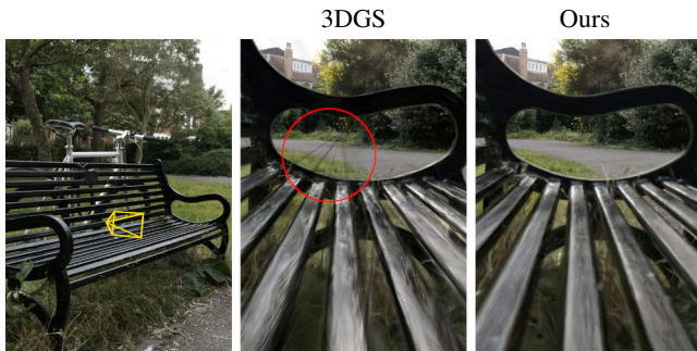
Figure 2: In 3DGS [KKLD23], Kerbl et al. use an affine approximation for projecting 3D Gaussians. Common benchmarks do not include viewpoints where this approximation matter is highlighted. Here, we demonstrate the benefits of our perspective-correct projection by comparing renderings from 3DGS and our method.
