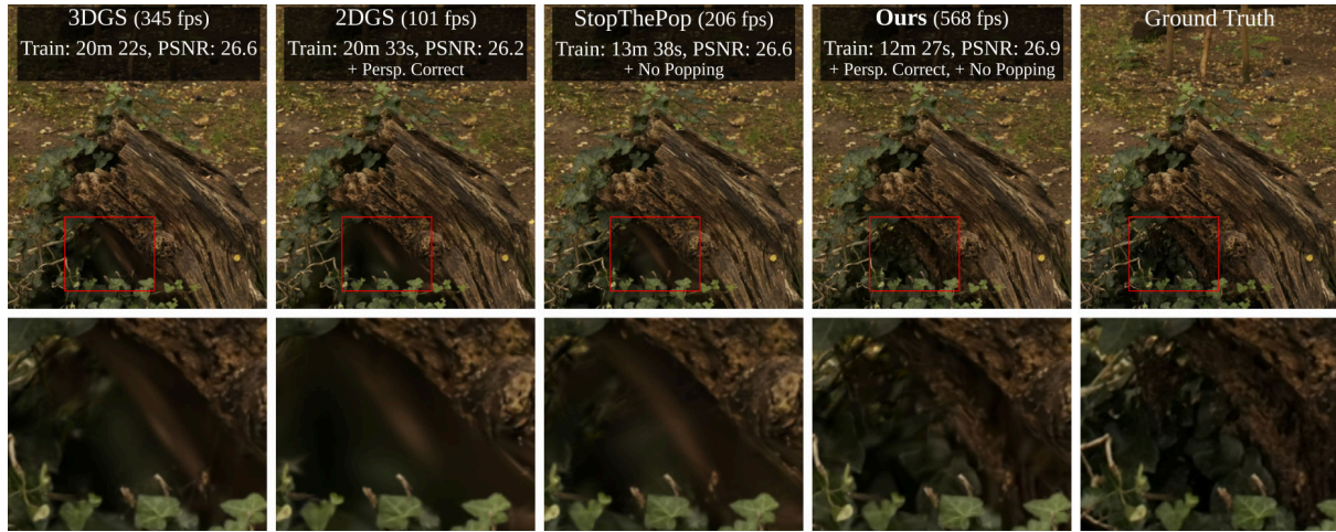
Figure 1: We present the first perspective and simultaneously geometrically accurate approach for real-time rendering of 3D Gaussian splats. Our temporally stable blending formulation based on hybrid transparency effectively removes the popping artifacts caused by the approximate, global sorting scheme of 3D Gaussian Splatting (3DGS) [KKLD23]. Additionally, we replace the approximate projection used in 3DGS with a novel, numerically stable formulation for evaluation of general 3D Gaussians along per-pixel rays to improve rendering quality. We also achieve a significant speedup compared to state-of-the-art approaches addressing these challenges [HYC*24, RSP*24], as our blending formulation only requires partial depth-ordering and our splat evaluation is well-suited for rasterization.
