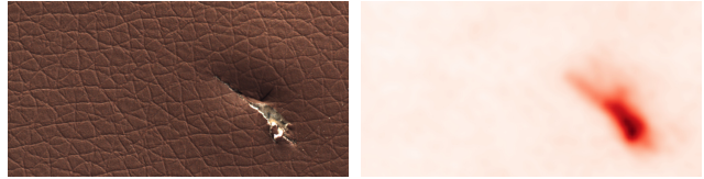
Figure 1: Anomaly localization. Left : input texture; right : anomaly map.
