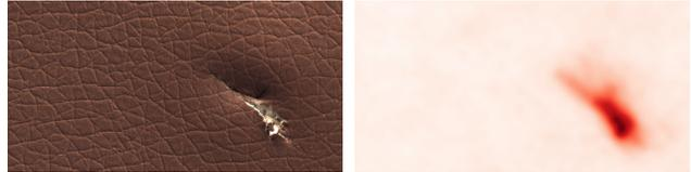
Figure 1: Anomaly localization. *Left:* input texture; *right:* anomaly map.
