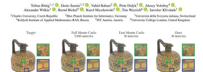
**Figure 1:** We propose a neural scattering compensation for 3D color printing. Comparing to a method which uses noise-free Monte Carlo simulation our technique achieves 300× speedup in the above case while providing the same quality.
