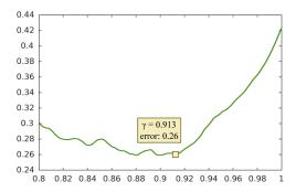
**Fig. 8.** The aggregate fitting error **y-axis** in dependence on the scaling factor  $\gamma \in [0.8, 1]$  **x-axis**. The error drops quickly between  $\gamma = 1$  and the global minimum at  $\gamma = 0.913$ , and then grows steadily again as  $\gamma$  tends to zero.
