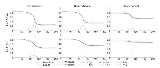
**Fig. 9.** Fitting results for the Vero PureWhite material. The plots show the best-fit profiles, as well as the corresponding gradient magnitude curves and adjacent dictionary records. Our fitting is robust to residual aberrations in the acquired data (e.g., see the blue channel at t = 0.5mm), yielding a reasonable match even in such cases.
