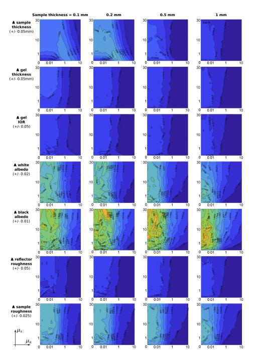
**Fig. 11.** Differential error analysis when perturbing seven selected salient dimensions (**rows**) of our measurement setup, evaluated densely for different combinations of  $\mu_a$  and  $\mu_s$  (in mm<sup>-1</sup>) and at 4 different sample thicknesses (**columns**). The deltas for each of the parameters are listed in the respective labels. The errors are computed by the profile distance metric (Eq. (2)), and normalized by the parameter deltas.
