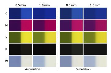
**Fig. 4.** Step edges captured through the printing materials  $\mathcal{M} = \{C, M, Y, K, W\}$  by our physical **left** and virtual **right** setups, at two different sample thicknesses. The images cover the area of  $20 \times 10$  mm (twice as wide as the cropped version our fitting operates with).
