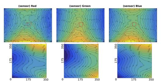
**Fig. 6.** False-color maps of the per-channel *relative* pixel intensity captured by our physical setup (denoised by an appropriate Gaussian filter). The iso-line spacing in the full images **top** is 1%, and 0.1% in the measurement region crops **bottom**.
