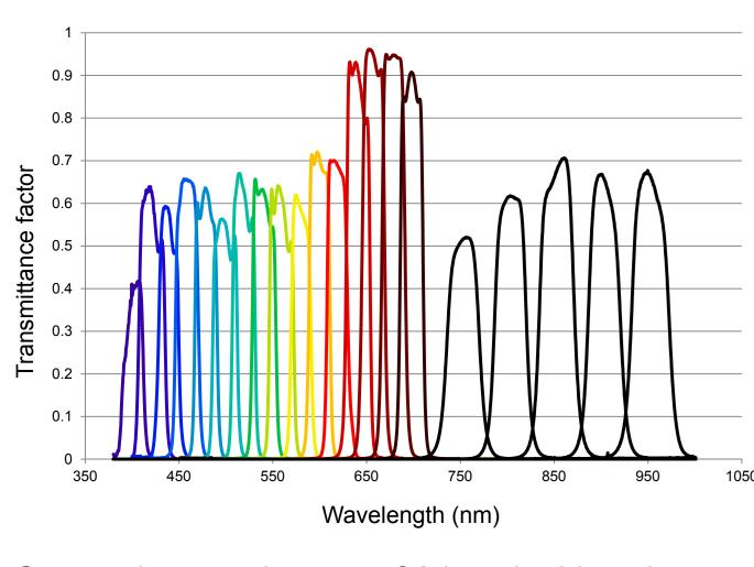
Spectral transmittance of 21 optical bandpass filters in the visible and NIR spectrum.
