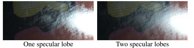
Figure 4: A single specular lobe (left) cannot capture heavy-tailed reflectance lobes of e.g. layered materials. A two-lobe model (right) matches observed behavior much better. All results use two lobes.
