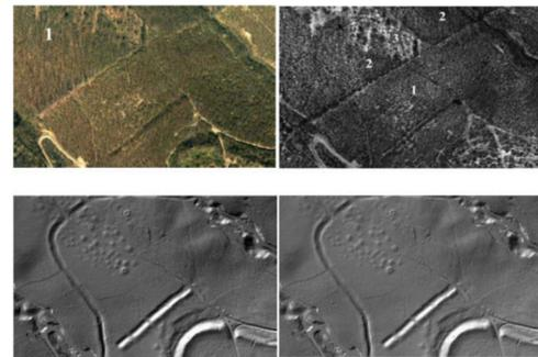
**Figure 26:** Analysis of airborne laser scanning data for archaeological sites identification. Top: aerial and intensity image of the studied area. Bottom: resulting DTM after processing, which shows possible archaeological sites once the information of forested areas has been removed. Courtesy of Doneus et al. [DB06] (Copyright Eurographics Association).
