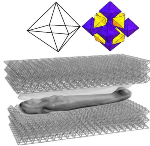
**Figure 24:** Geometric analysis for packaging applications. Top: the octahedron, which is the basic unit that has been used to build the 3D printed package. Bottom: The final structure ready to print. Courtesy of Sá et al. [SEG\*12] (Copyright Eurographics Association).
